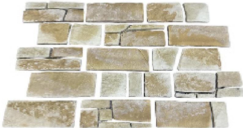
**Installing with Dry Joint:** Please ensure either the wall or adhesive are a dark colour before starting. This can be done by purchasing a dark tile adhesive or tinting adhesive mortar with black oxide. This will help cast a shadow between stones giving a deep solid dry stone look. Take time once the pattern is laid to cut thin stones to fill small gaps between the larger joints. This is very important, it will break up the pattern and provide the perfect hand crafted stone masonry look.
